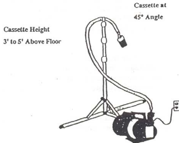
FIGURE 12-1 Proper Sampling Technique
